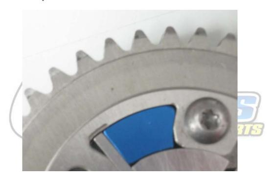
12. The torque for the bolts is 145 in lbs. We recommend using a small dab of blue thread locker on each bolt.
